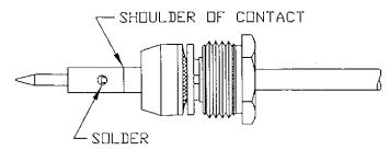
3. SLIP INSULATOR OVER DIELECTRIC, SLIDE CONTACT ONTO CENTER CONDUCTOR UNTIL THE SHOULDER IS FLUSH WITH THE INSULATOR, PRESS FIRMLY IN PLACE AND SOLDER AS SHOWN.
