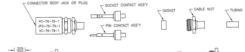
PLACE TUBING, CABLE NUT, AND GASKET OVER CABLE OUTER JACKET. TRIM CABLE TO DIMENSIONS SHOWN TO EXPOSED CENTER CONDUCTOR.
